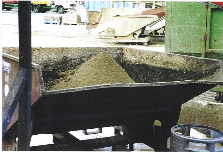
Cake and Centrate Produced by Centrifuging Potato Effluent 35% DS
