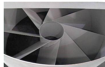
Top view Centri-Flow tank and circular weir
