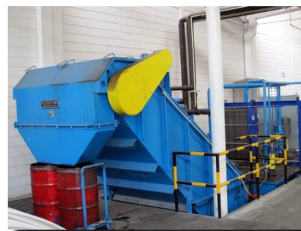
240 GPM (912 LPM) Filter System for 2-Wire Rod Breakdown Machine
