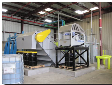
350 GPM (1325 LPM) Filter System for Two (2) Rod Breakdown Machines
